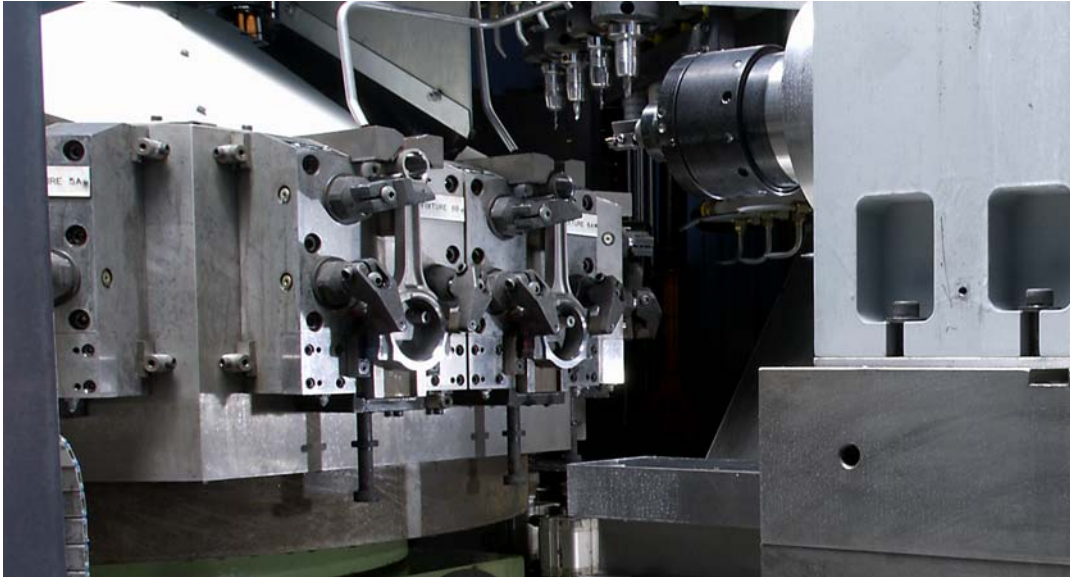
Single clamping on the ATS Turn 6 LC CNC dial machine provides high accuracy and repeatability for the high-volume machining of these powder metal connecting rods.
