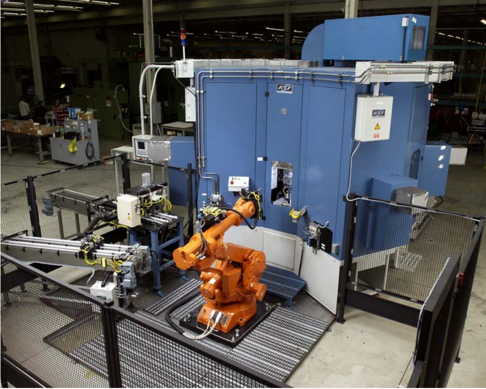
Automatic load/unload on the ATS Turn 6 LC, incorporating a twin-lane conveyor and an ABB 4400 Series robot.
