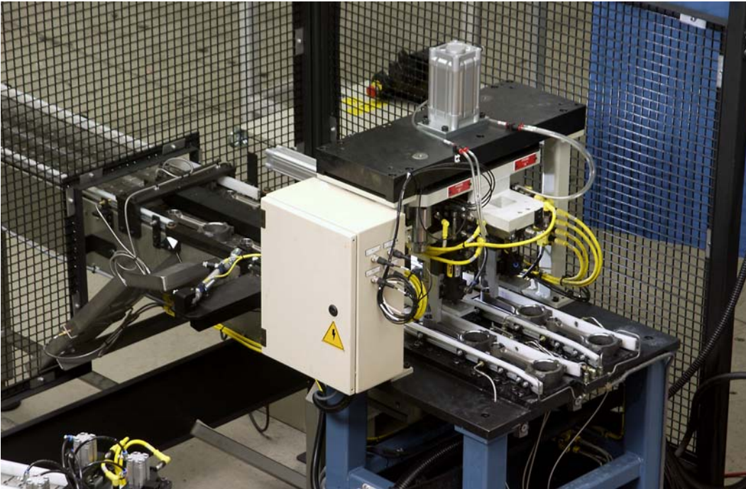
Close-tolerance machined features on powder metal connecting rods are automatically measured, and the data sent to the controller which computes the tool movement.
