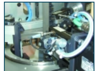
Three winding needles, arranged at 120° in a circle
